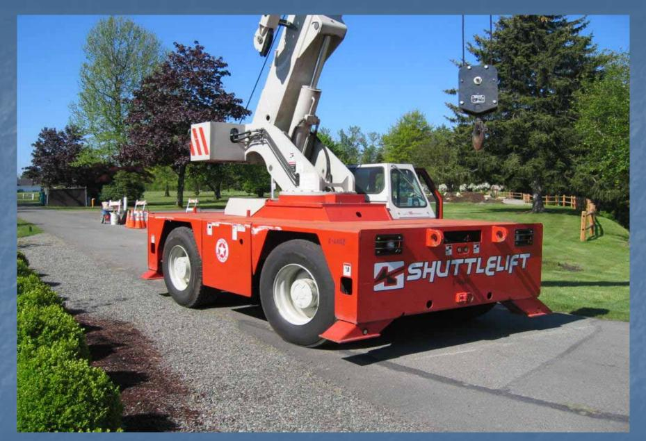
This crane has a deck on the front to set the columbarium while moving into position.
